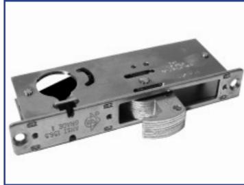
50-06-100 Lock Body, Hook Type Narrow, 1-1/8" Backset
